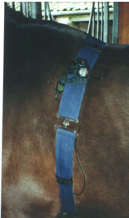
Figure 3: Receivers for Polar Vantage NV located dorsolaterally on the surcingle between the two transmitter electrodes
